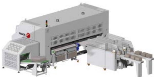
● Stohovač malého prádla s 2 drahami + SMARTY. / Small pieces back collector 2 lanes + SMARTY.
